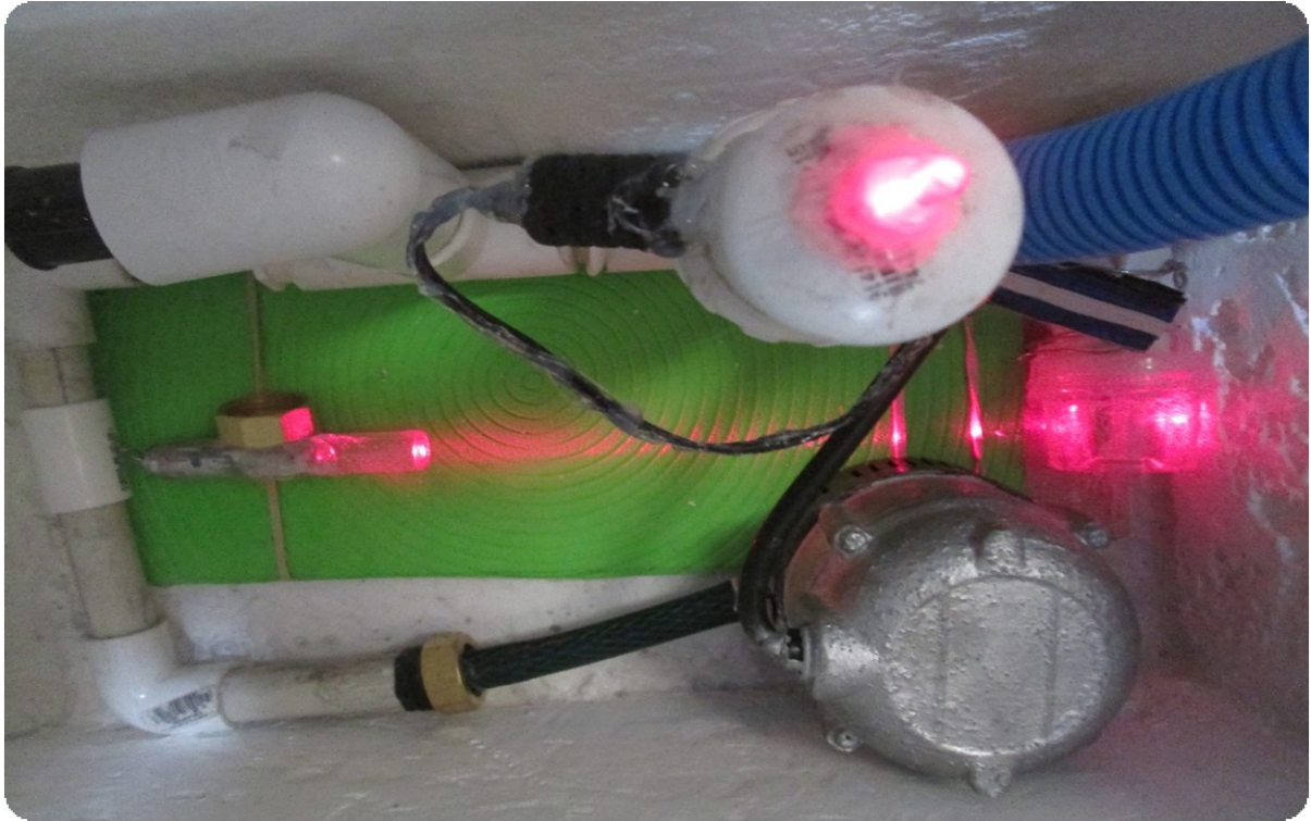
PHOTO 3. LASERS AND ROBOT MOTOR submerged in water.
