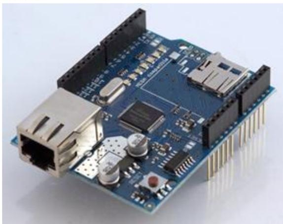
Figura 2.11 Arduino Ethernet Shield.
