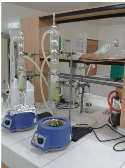
**Figura N°24.** Aparato Soxhlet
