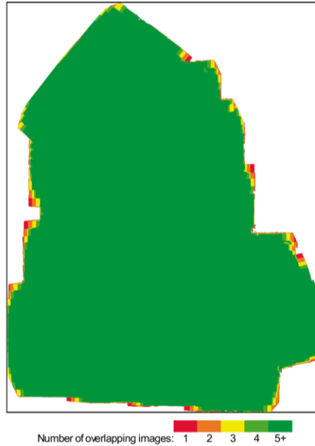
Figure 4: Number of overlapping images computed for each pixel of the orthomosaic. Red and yellow areas indicate low overlap for which poor results may be generated. Green areas indicate an overlap of over 5 images for every pixel. Good quality results will be generated as long as the number of keypoint matches is also sufficient for these areas (see Figure 5 for keypoint matches).
