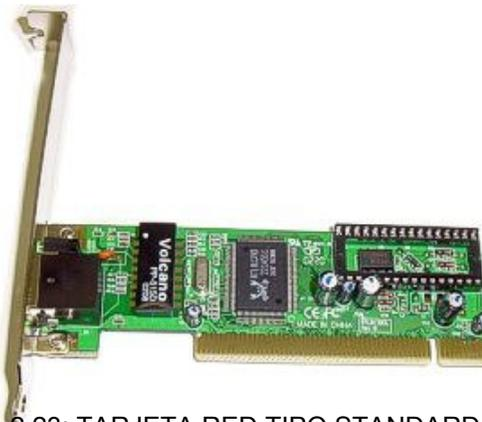
FIG. 2.23: TARJETA RED TIPO STANDARD
