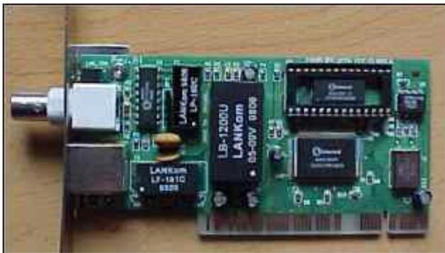
FIG. 2.22: TARJETA RED CON CONECTOR BNC
