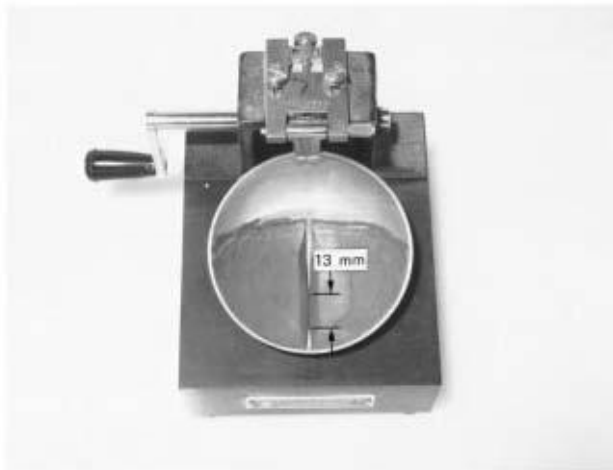
FIG. 7 Soil Pat After Groove Has Closed
