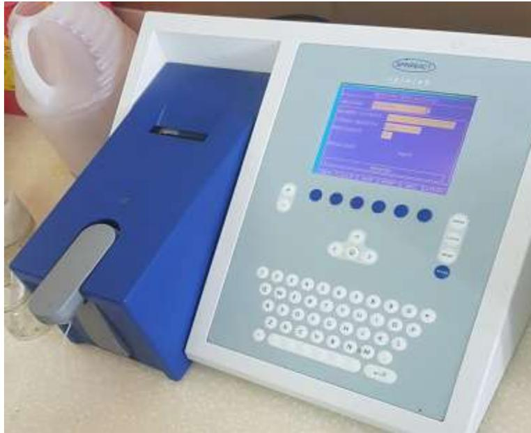
**FIGURA 1: EQUIPO DE LECTURA PARA LAS MUESTRAS DE GLUCOSA BASAL EN AYUNAS Y TOLERANCIA ORAL A LA GLUCOSA (ESPECTROFOTÓMETRO)**
