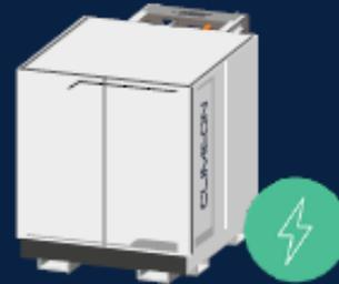
**THE HP 150 MODULE** is the building block of the Climeon Heat Power System, which converts low-temperature heat into clean electricity. Using the principles of the Organic Rankine Cycle, but at much lower pressure levels, the system is designed for unmatched efficiency within the operating temperatures.
