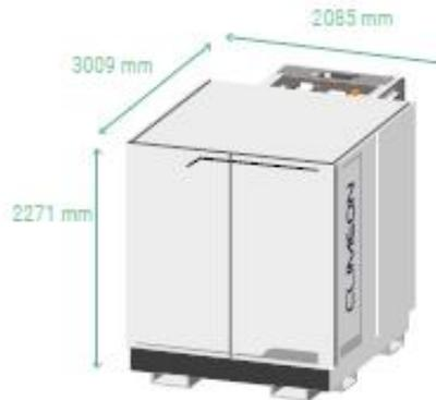
Please note: Space of 150mm in front, 50mm above, and 60mm behind is needed around the module. 50mm is recommended between modules, when more than one module is present.
