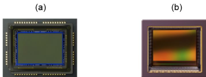
Figura 2.2: Cámaras modernas de semiconductores: (a) CCD (recuperada: https://www.imaging-resource.com/PRODS/D3000/ZD3000SENSOR-LG.JPG ), (b) CMOS (recuperada de: https://www.dataray.com/blog-cmos-vs-ccd-overview.html )
