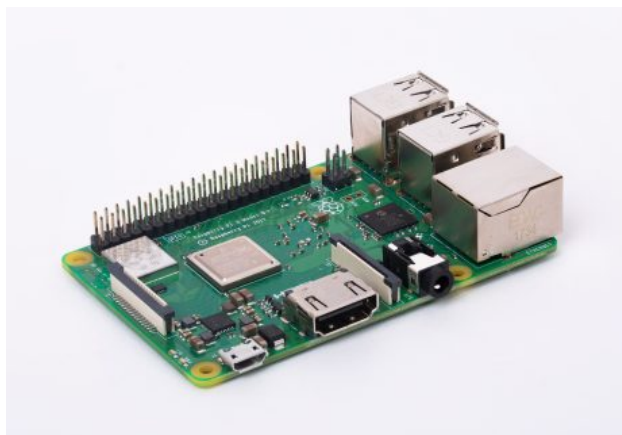
Figura 2.22: Raspberry PI 3 Modelo B+. Recuperada de: https://www.raspberrypi.org
