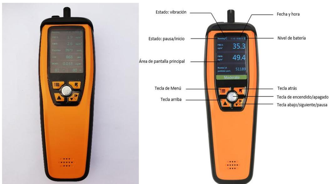
Figura 4.3: Dispositivo Elitech Temtop M2000 (*Elitech Technology Inc, 2020*)
