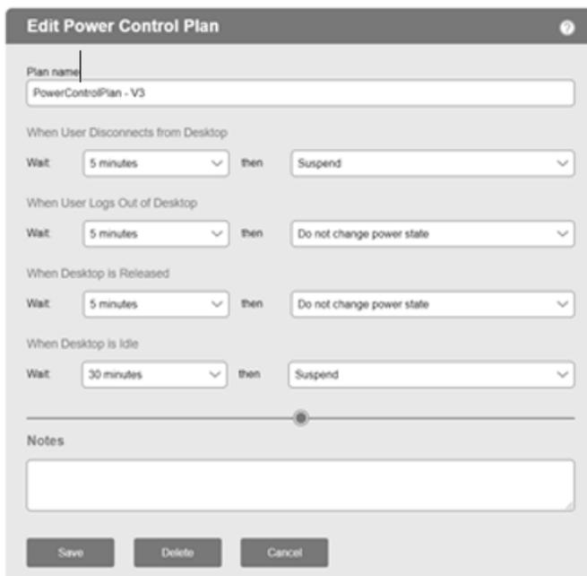
Figura 138. Power control plan
