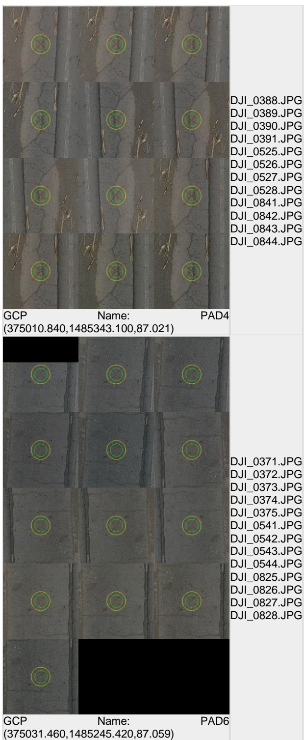
Figure 7: Images in which GCPs have been marked (yellow circle) and in which their computed 3D points have been projected (green circle). A green circle outside of the yellow circle indicates either an accuracy issue or a GCP issue.
