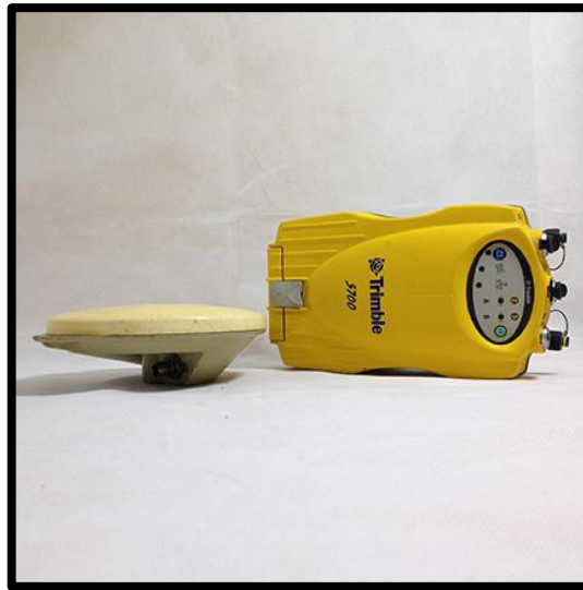
Figura 3.2 Antena Zephyr y receptor Trimble 5700
