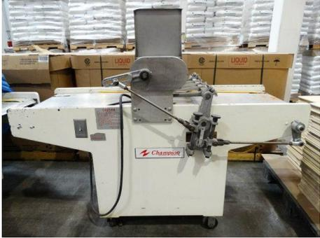
A white industrial cookie dropper machine, model Champion 65-S, is shown in a bakery or warehouse setting. The machine has a large hopper on top, a roller mechanism, and a cutting head. It is mounted on four casters. The background shows stacks of cardboard boxes and a concrete floor. |
