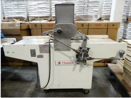
A white industrial cookie dropper machine, model Champion 65-S, is shown in a bakery or warehouse setting. The machine has a hopper on top, a mixing mechanism, and a dispensing nozzle. It is mounted on four casters for mobility. The background shows stacks of boxes and other bakery equipment. |
