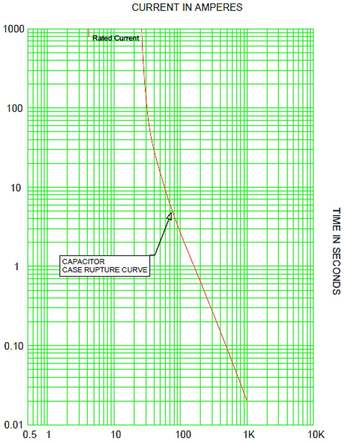
CAPACITOR.tcc Ref. Voltage: 4160 Current Scale x10<sup>4</sup>
