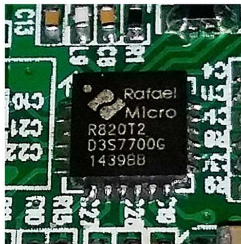
The R820T2 on a RTL-SDR V3
