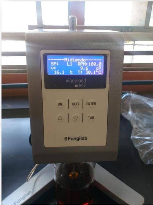
**Figura 26.** Viscosímetro "Fungilab" Viscolead ADV H
