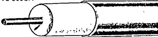
Copper clad aluminum center conductor; expanded polyethylene dielectric; solid aluminum sheath; center conductor 0.111" (2.82mm) nominal; nom. O.D., 0.500" (12.70mm).
