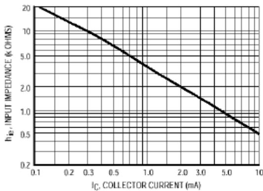
Figure 13. Input Impedance
