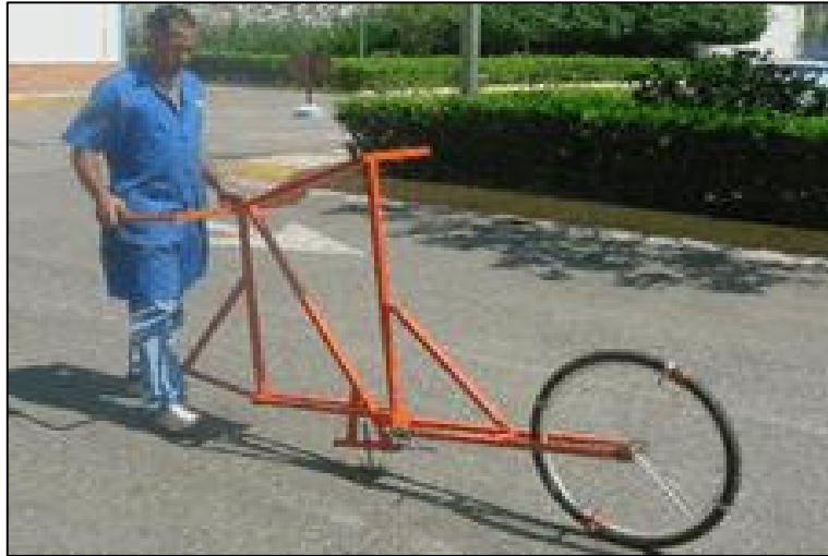
Fig. 2.8 MERLIN (Machine for Evaluating Roughness using Low cost Instrumentation)
