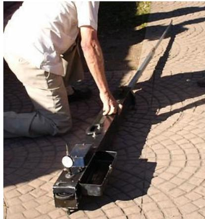
**Fig. 3.5 Viga Benkelman**
