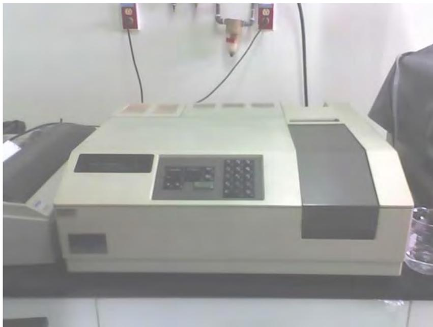
**Fig. 16 ESPECTROFOTOMETRO UV-VISIBLE**
