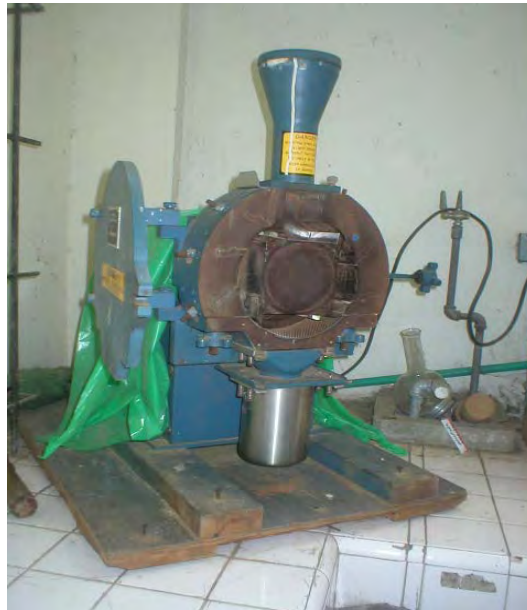
Figura № 13. Molino Thomas Willey Laboratorio Mill model 4.
