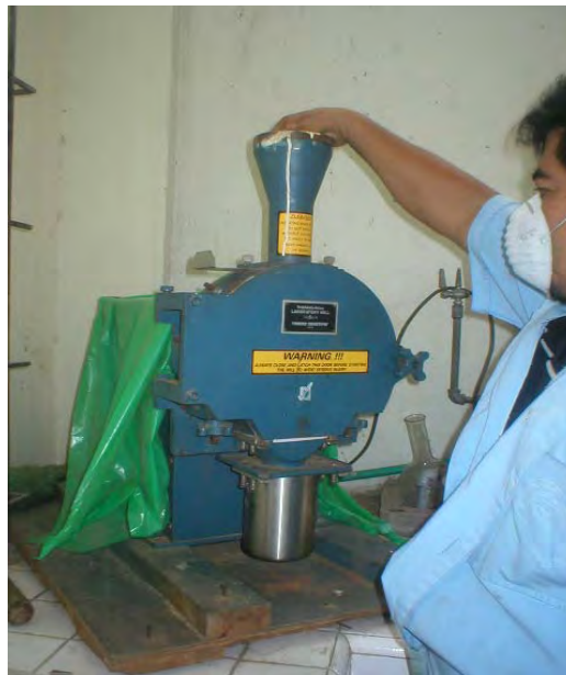
Figura № 13. Molino Thomas Willey Laboratorio Mill model 4.
