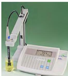
Fig. 23. *pHmetro Mettler Toledo.*
