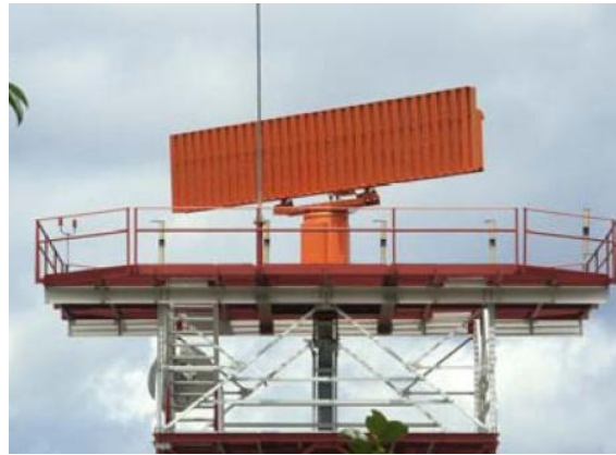
Figura 1.6: MSSR INDRA IRS-20MP/S
