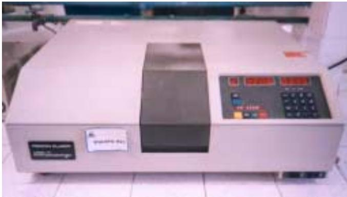
Fig.No.8 Espectrofotómetro Ultravioleta-Visible Perkin-Elmer Lamda 1 A.
