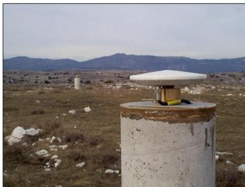
**Figura 3.18 Antena GPS.**
