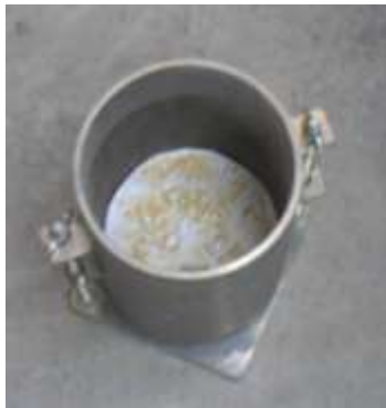
Fig. 3-5: Moldes de Base Perforada
