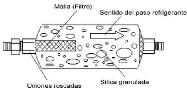
FIGURA 38 ESTRUCTURA INTERNA DEL FILTRO
