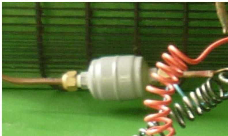
FIGURA 52. FILTRO SECADOR FLARE DE 1/4" O-D32 SPORLAND
